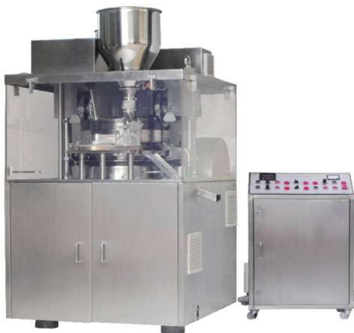
Fig.6: 16 STATION TABLET PUNCHING MACHINE
